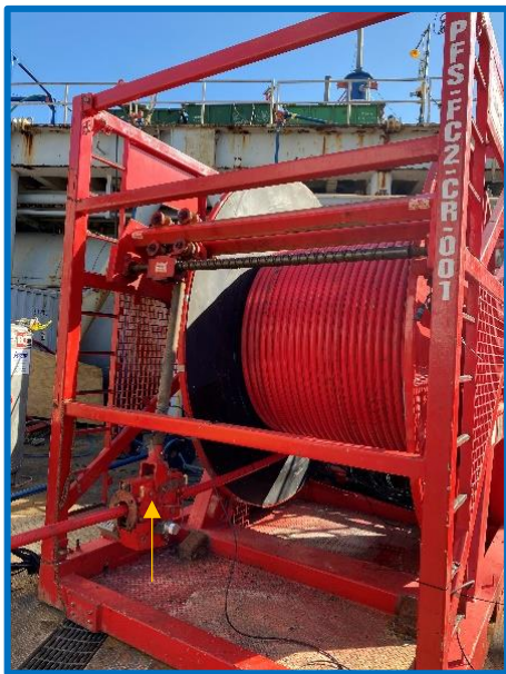
Incident 1: The spot where the contractor's right thumb was pinched between the ball valve and the horse head.
