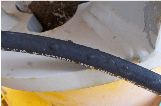
Incompatible hydraulic hose blistered during use.
