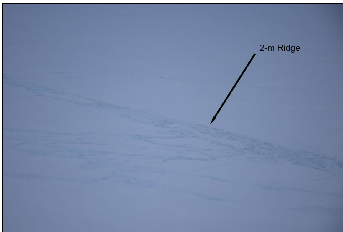
Plate 5-12. Undeformed First-Year ice with 2-m Ridge in Camden Bay Prospects 23 nm North of Mary Sachs Entrance (looking north on February 22, 2020)
