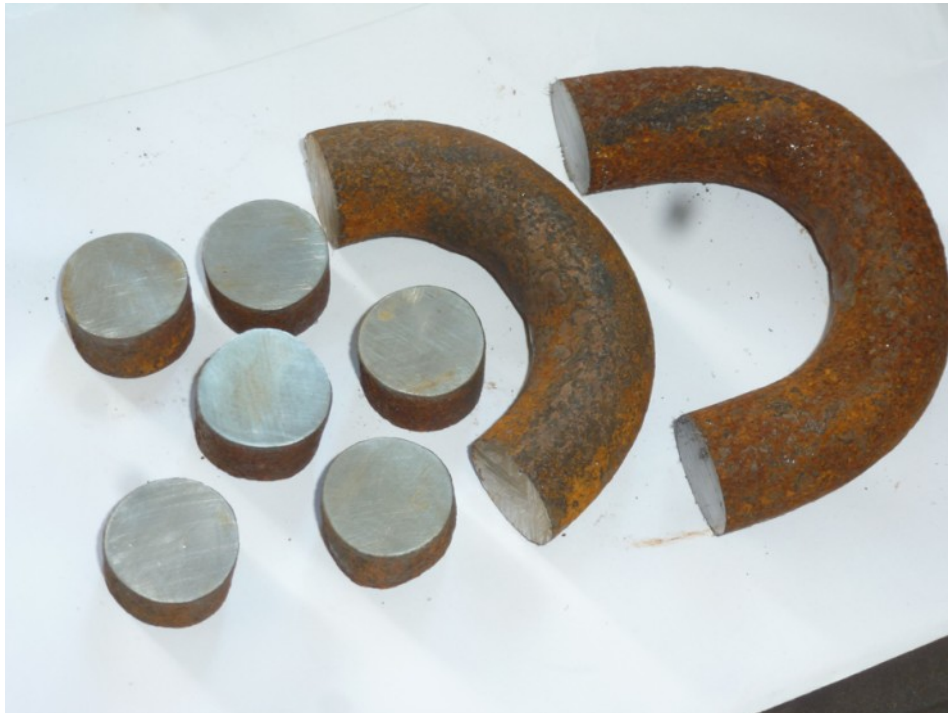
Figure 24: Hardness specimens cut from a chafe-zone link.
