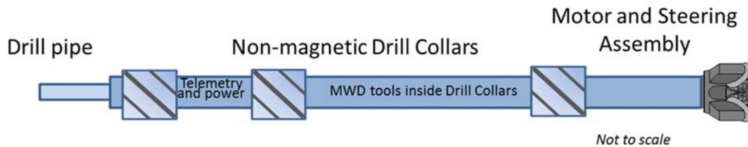
Figure 14: Bottom Hole Assembly showing location of MWD Tools
