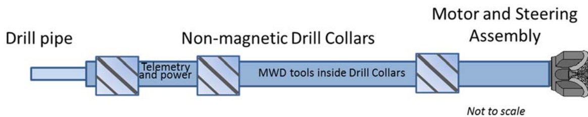
Figure 11: Bottom Hole Assembly showing location of MWD Tools
