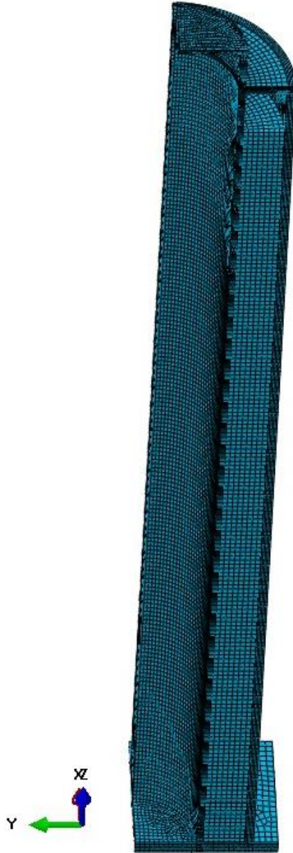
Large scale FEA element mesh
