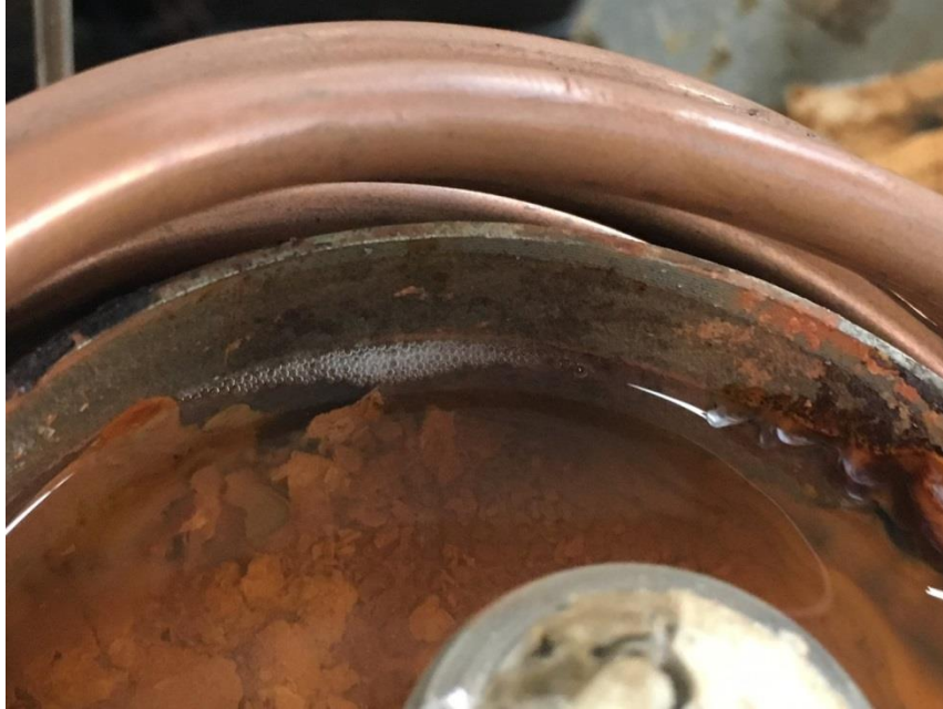
Figure 69 Thermal shock test – failure on outer radius of cement
