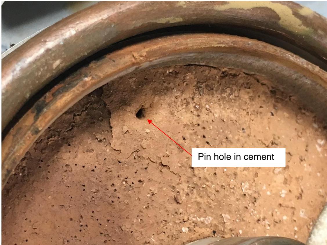
Figure 68 Thermal shock test fail – pre-mature failure
