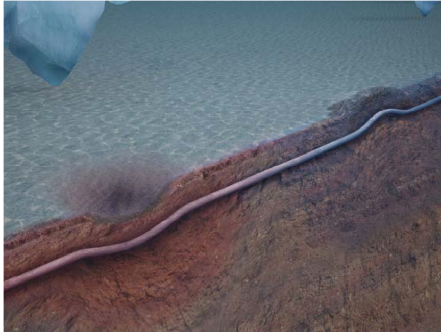
Figure 4-3: Thaw Settlement and Frost Heave
