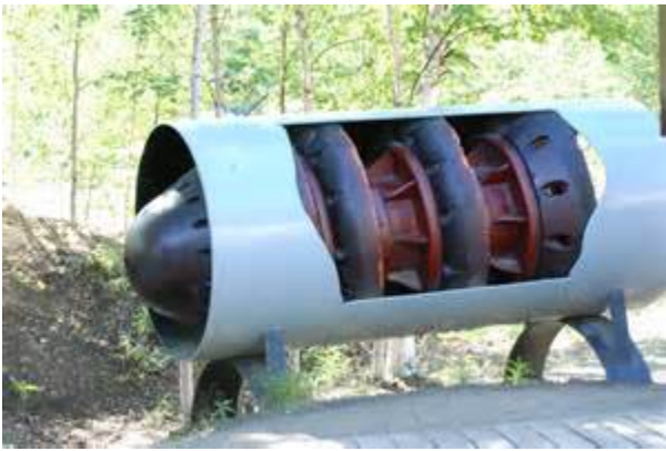
Exhibit 1: Example Pig Used in the Trans-Alaska Pipeline 1
