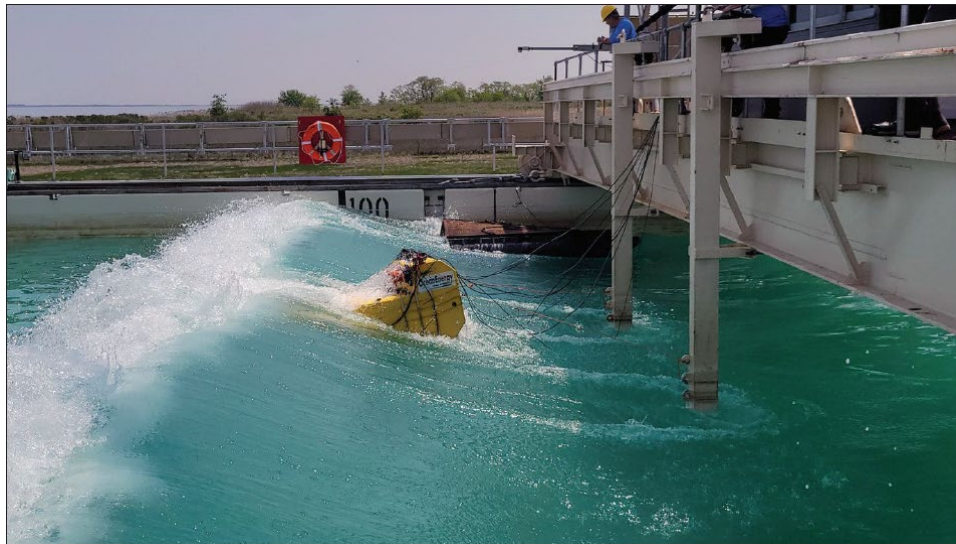
Figure 6. On the Ohmsett tank, OceanEnergy's 1:15 floating oscillating water column wave energy converter was studied for operational and structural performance. From Fall/Winter 2022 Ohmsett Gazette. "Wave Energy Evaluation." Page 1.
