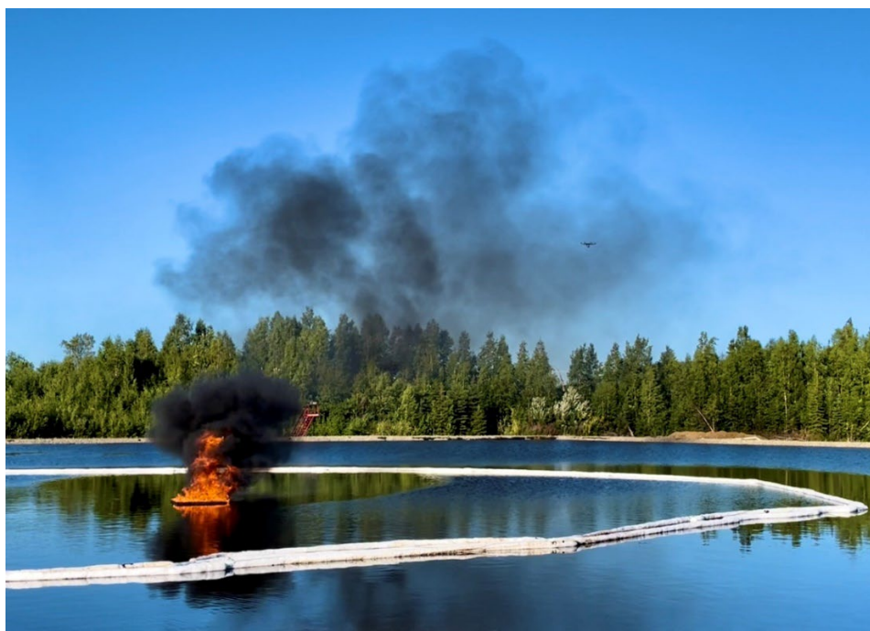
Figure 3: A drone equipped with chemical sensors samples the smoke plume emitted from a burn of Alaska North Slope crude oil at the Poker Flat Research Range in Chatanika, Alaska. This was one of several test burns conducted in early August 2022 to better understand the fate and transport of smoke plumes from these types of operations. This BSEE-led project was coordinated between key stakeholders including the EPA’s Office of Research and Development, Office of Emergency Management, and Region 10; the U.S. Geological Survey’s National Uncrewed Systems Office; NOAA’s Air Resources Laboratory; the USCG Pacific Strike Force; the University of Alaska Fairbanks’s Poker Flat Research Range and International Arctic Research Center Uncrewed Aircraft Systems Team; and Alaska Clean Seas. (Photo from Karen Stone, BSEE)
