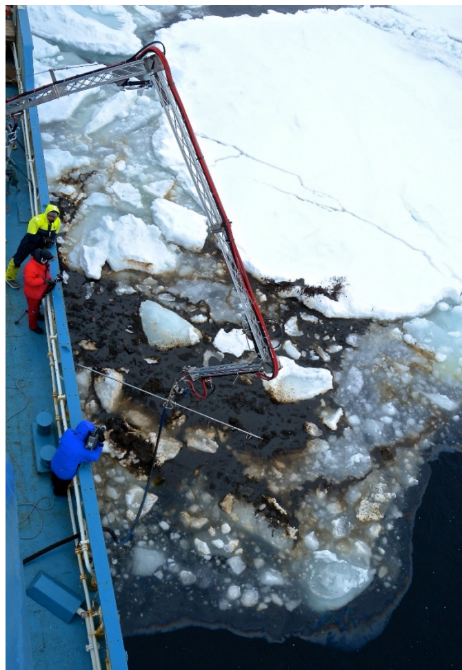
Figure 19. View of the specialized dispersant application arm developed and tested in the SINTEF Oil in Ice JIP in 2009 in the Norwegian Barents Sea with the aim to improve the targeting and delivery of dispersant to isolated oil patches among ice floes (Photo: D. Dickins).
