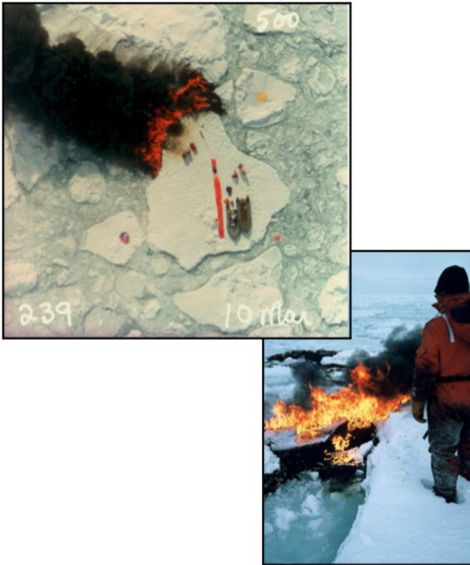
Figure 21. Aerial and surface views of burning crude oil spilled in slush between floes during the 1986 Canadian East Coast” Oil in Pack Ice” experiment (Buist and Dickins, 1987) (Photos: L, R: R. Belore, D. Dickins).
