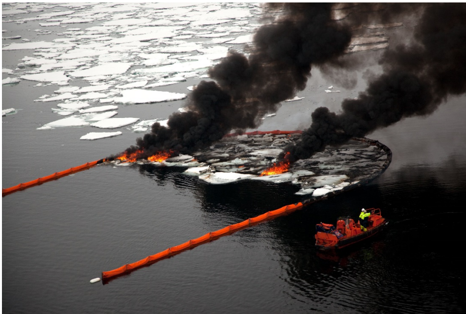
Figure 22. Burning crude oil spilled into a field of small ice cakes collected in a fire-resistant boom – Norway 2009 (Potter et al., 2012).
