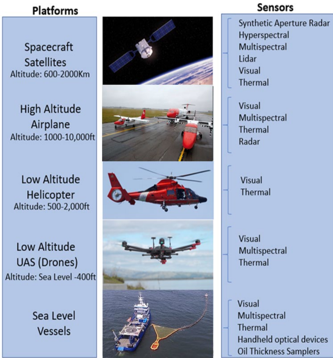
Figure 3. Representative platforms and sensors used for oil spill remote sensing monitoring. Platforms are classified by altitude and coverage.
