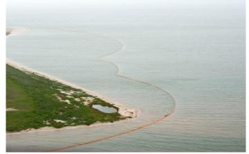
Figure 15. An example of a nearshore boom deployed (Source: USCG).
