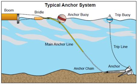
Figure 14. Typical boom anchor system (Source: Spill Tactics for Alaska Responders, 3/2014).
