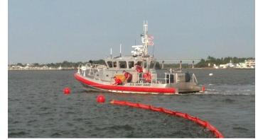
Figure 16. A nearshore deployed boom being recovered (Source: USCG).
