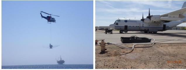
*Figure 8.* Helicopter exercising simulated dispersant application with bucket sprayer (Source: BSEE).
