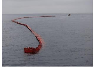
Figure 1. Small boat deploying curtain boom offshore (Source: BSEE).
