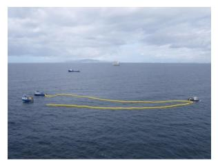
*Figure 3.* Two vessels deploying containment boom in V-shape while third vessel deploys a free-floating brush skimmer in apex of configuration (Source: BSEE).
