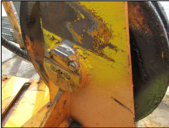
Abraded main line carrier sheave side plate and pin boss.
