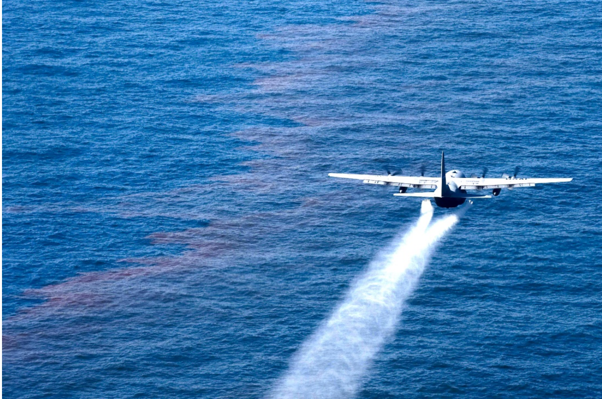
Figure 14. C-130 Hercules from the Airforce Reserve Command's 910 th Airlift Wing drops dispersant as part of the Macondo Response Effort.
