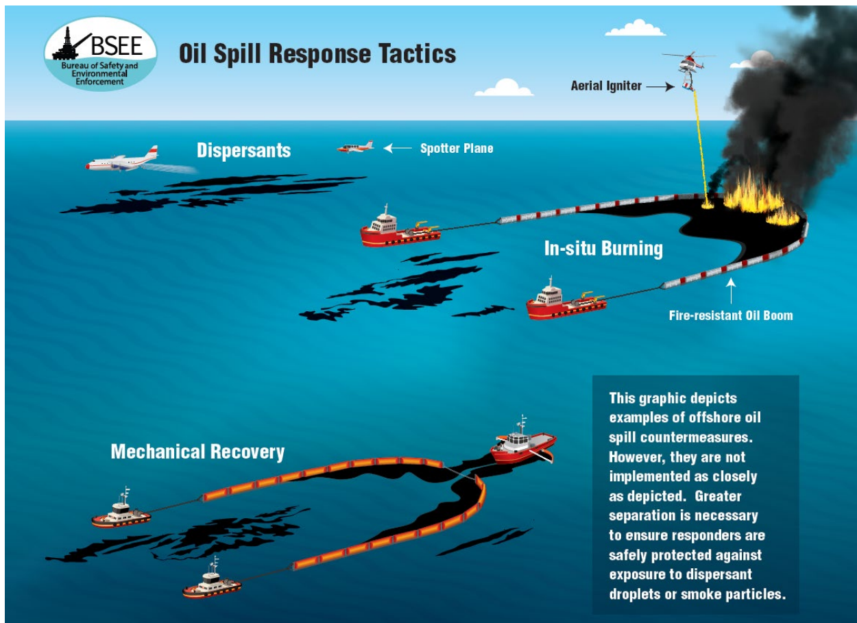
Figure 1. Oil Spill Response Tactics that could take place in different zones of the FORD.
