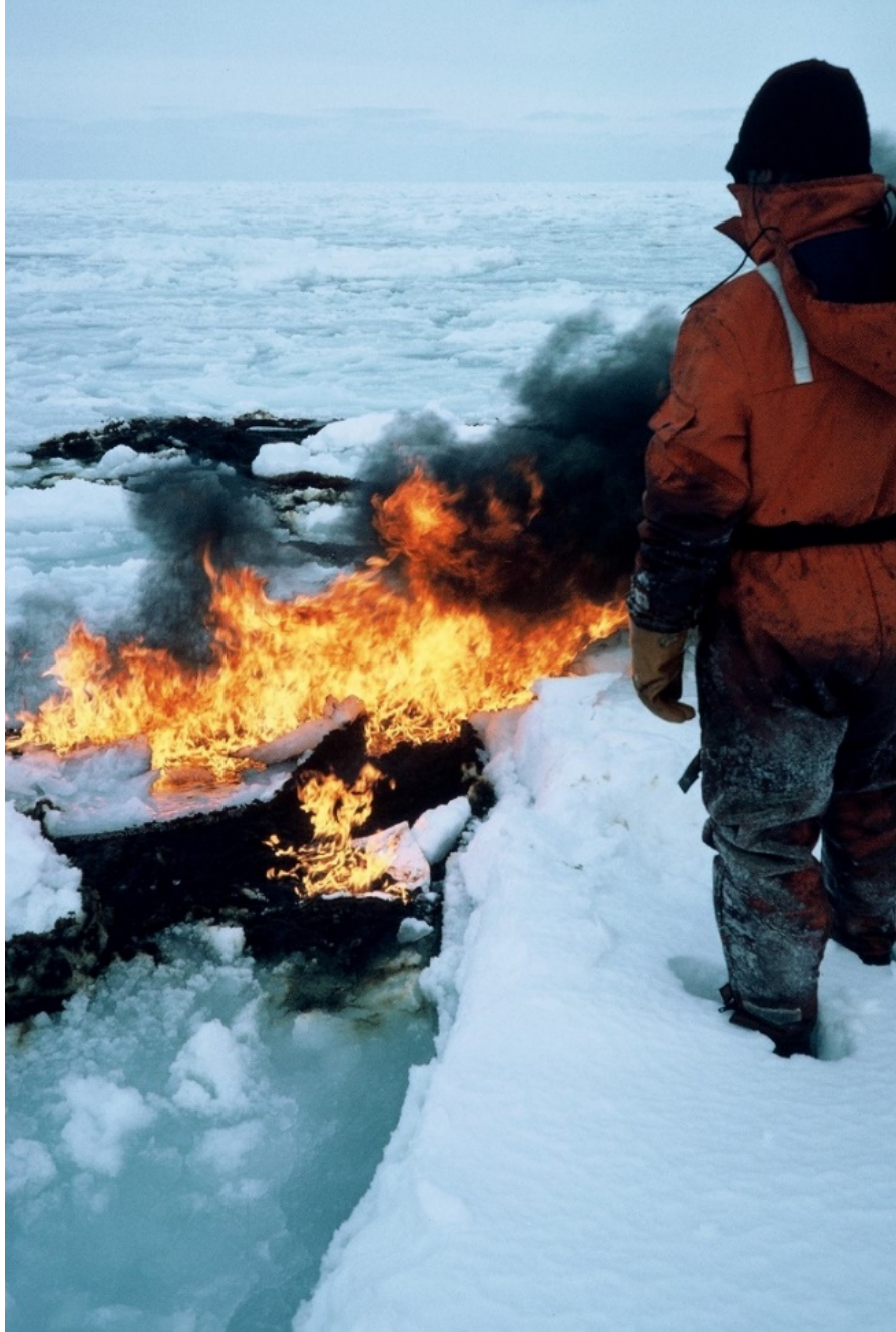
Figure 15. Burning crude oil in slush between ice floes during the 1986 Canadian East Coast “Oil in Pack Ice” experiment. Ref. Buist and Dickins, 1987. Photo: D. Dickins.
