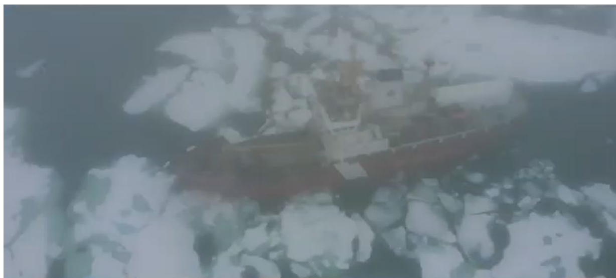
Figure 13. Example showing the difficulty of operating UAS (drones) In the Beaufort Sea and the challenges for detection of oil spills from aerial platforms during foggy conditions.
