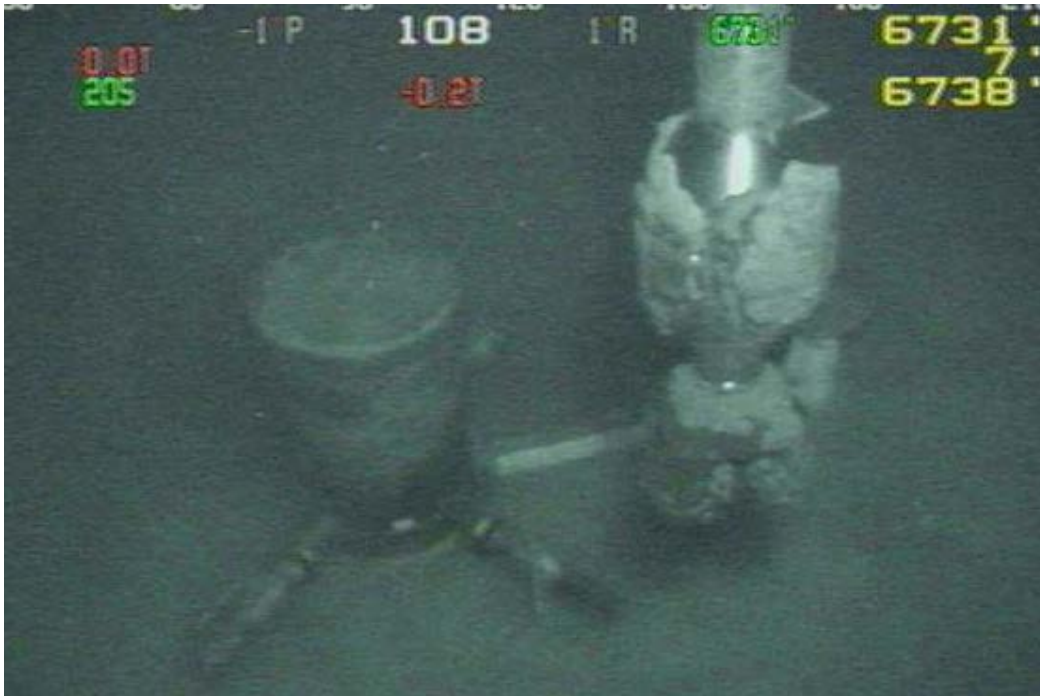
Figure 6-7: Balled Stabilizer when Drilling Shallow Sediments prior to Running Marine Riser
