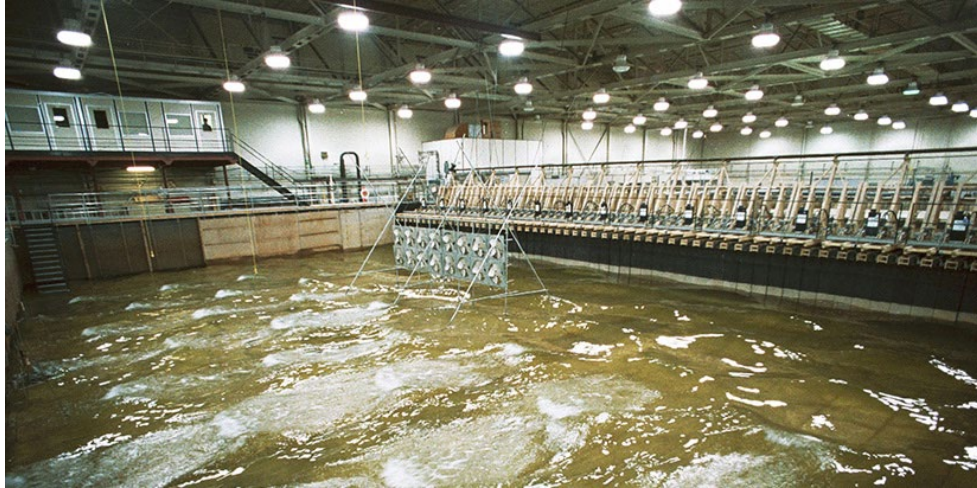
Figure 4: NRC (Canada) Ottawa Multidirectional Wave Basin
