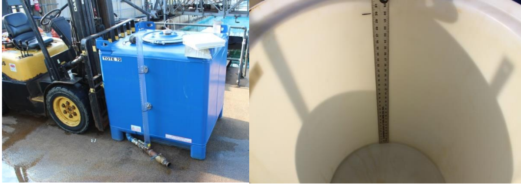
Figure 9 – Tote for Dispensing Test Oil and Inside View of Calibrated Recovery Tank
