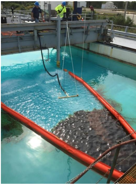
Figure 6 – Containment Boom and Oil Distribution Bar
