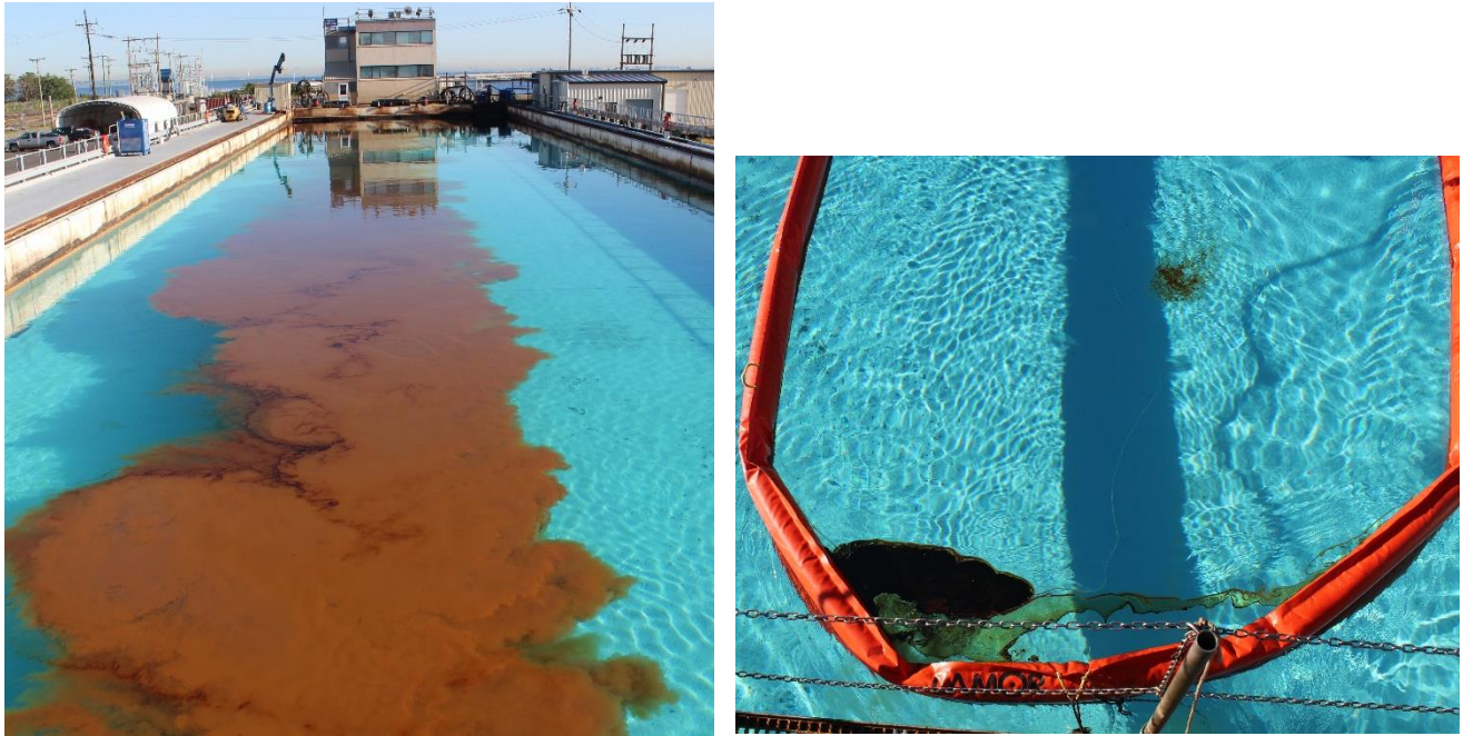
Figure 15 – Oil Dispersed Behind Boom (left) and Remaining after DOR 1:50 test (right)
