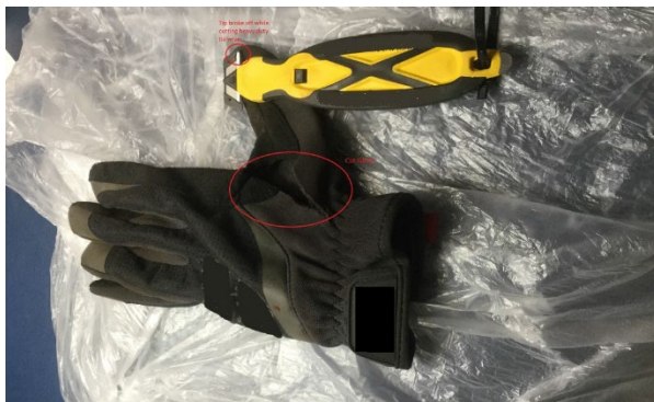
Figure 1 - Damaged alternative cutting device and cut glove.
