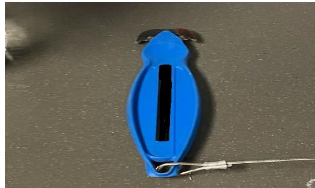
Figure 2 - Exposed blade on alternative cutting device.
