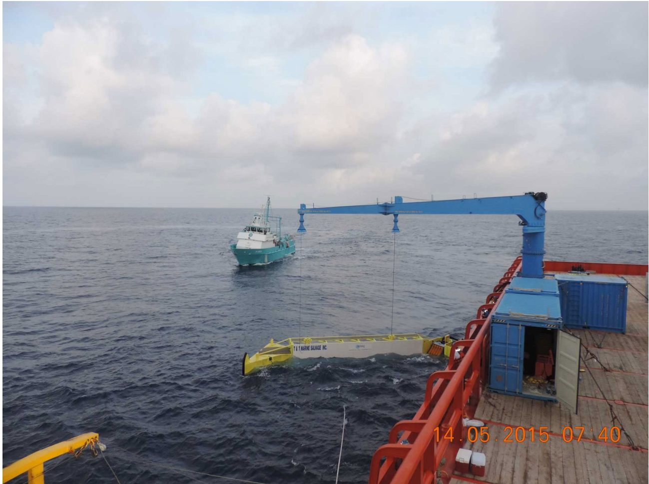
Figure 11. Example of a Rigid Arm System. (Photograph courtesy of Clean Gulf Associates, KOSEQ Rigid Sweeping Arms - Clean Gulf Associates ).
