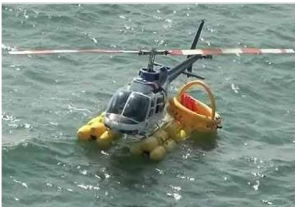
Figure 7. Floats and raft deployed
