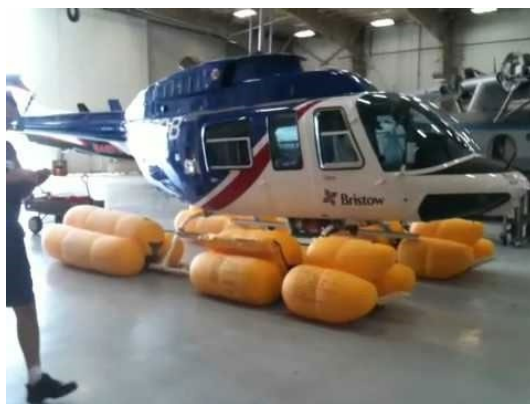
Figure 8. Test of float system deployment
