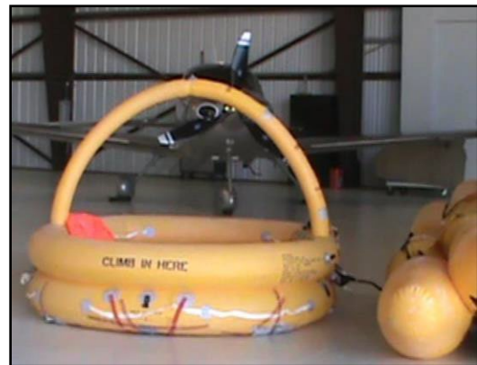
Figure 6. External life raft deployed.
