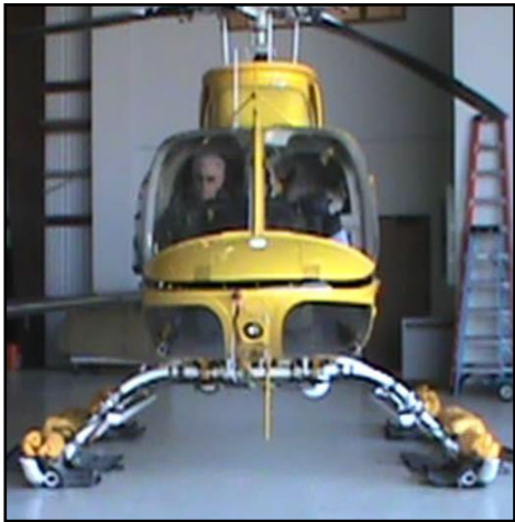
Figure 3. Normal float configuration
