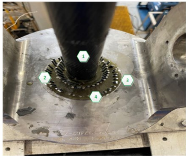
Actual Failed Termination of the ROV Umbilical and Example of Correct Strand Centering Distribution.
