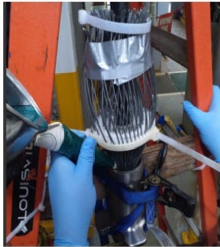
Figure 2: Inverted Resin Fill Cone and Armor Strands.
