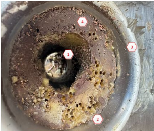
Actual Failed Termination of the ROV Umbilical and Example of Correct Strand Centering Distribution.
