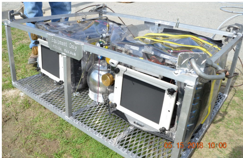
Figure 2-2. U.S. EPA's emission instrument system (the "Flyer") mounted on an aluminum skid.
