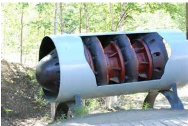
Exhibit 1: Example Pig Used in the Trans-Alaska Pipeline 1
