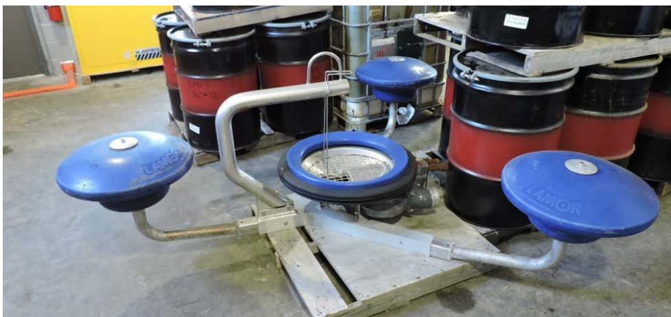
Figure 4 Lamor LWS 500\GTA50 Weir Skimmer
