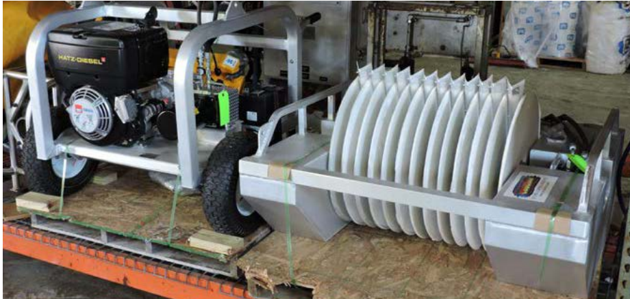
Figure 7 Crucial C-13/24 Coated Disc Skimmer
