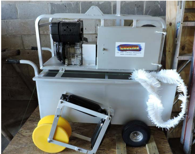
Figure 3 Crucial C-14d Mop Wringer System
