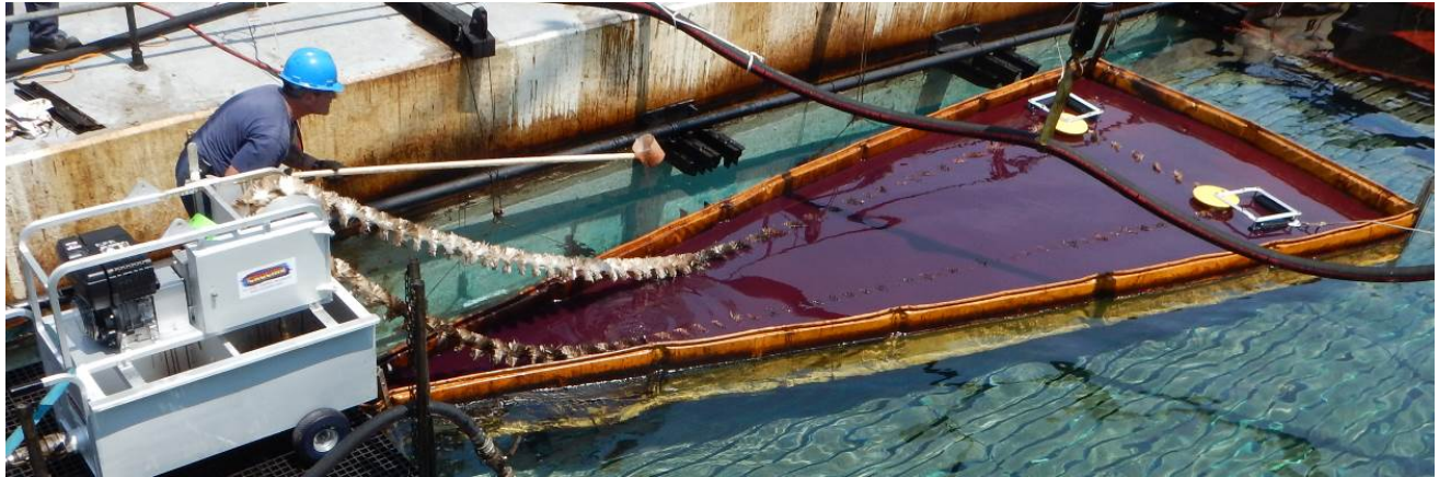
Figure 11 Crucial C-14d Mop Wringer System
