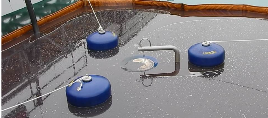
Figure 12 Lamor LWS 500\GTA50 Weir Skimmer
