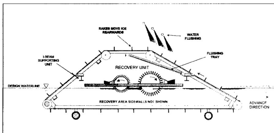
Fig. 10. LGB with flushing system and recovery unit.
