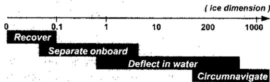
Fig. 1. Response method according to ice dimensions.
