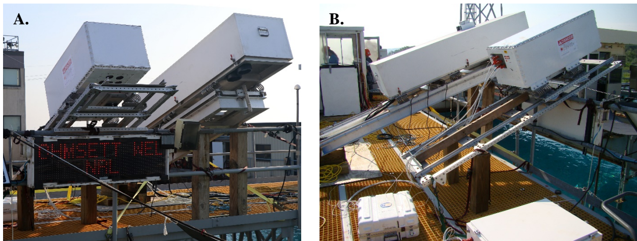
Figure 2. NRL LiDAR systems deployed on the railing on the auxiliary bridge (facing the main bridge). SLOP on the left, TURBOL on the right. A. Front view. B. Rear view.
