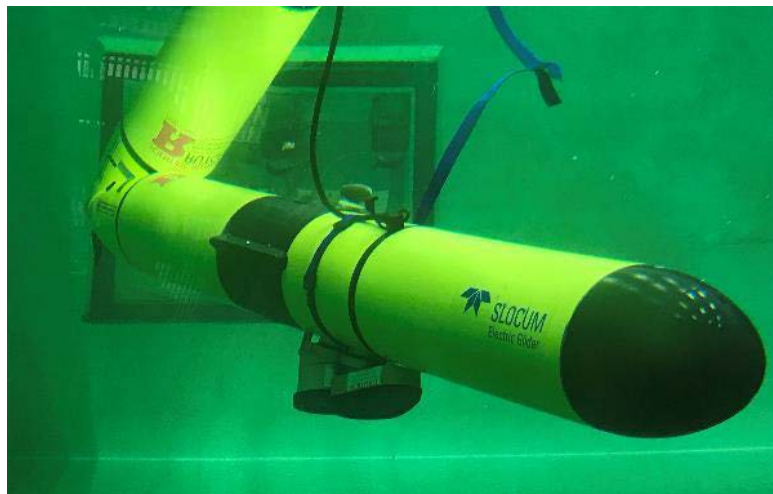
Figure 7. Multifrequency AZFP integrated into Slocum glider (transducer protruding below).
