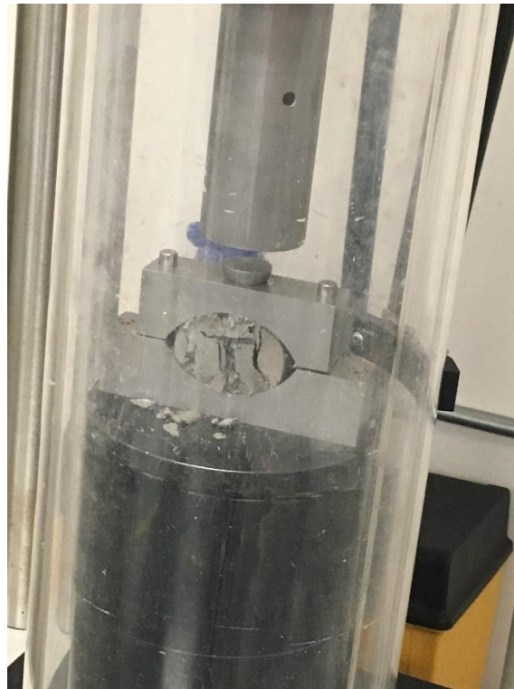
Tensile testing – Indirect Tension – “Brazil Test”
