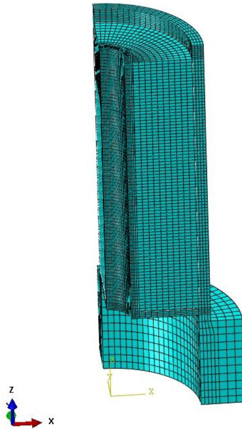
Small scale FEA element mesh
