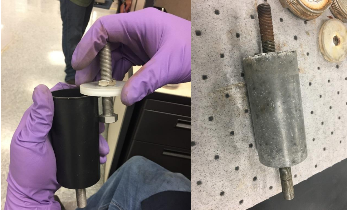
Figure 57 Tensile testing – direct test mould and test sample
