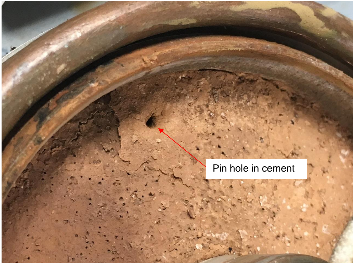
Figure 68 Thermal shock test fail – pre-mature failure
