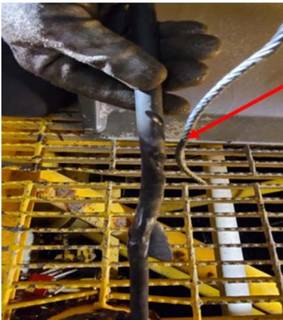
*A frayed SRL cable that made contact with metal grating.*
