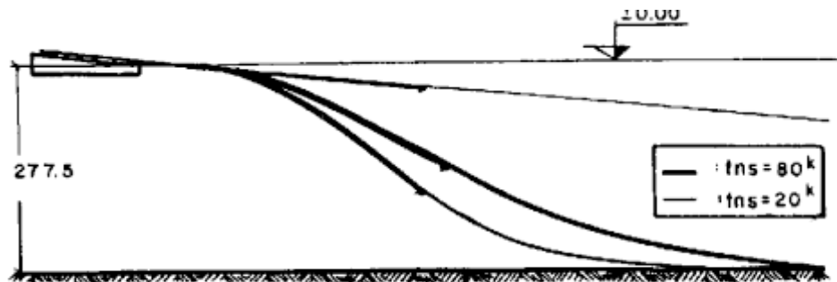
Figure 3.3: The deformed configuration of a pipeline during construction.[3]
