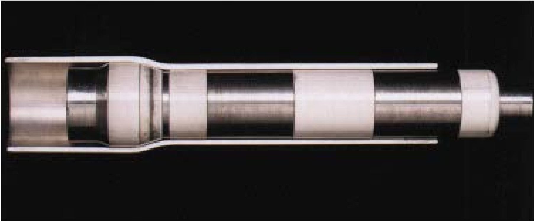
Fig. 1—Cross-section of partially expanded pipe with mandrel.
