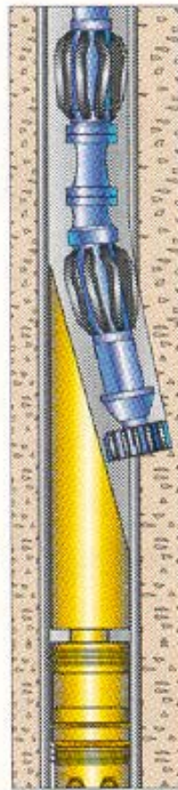
Shear bolt & start window cutting
