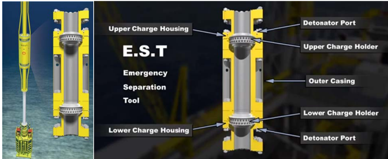
Figure 10.7: Components of Emergency Separation Tool [39]
