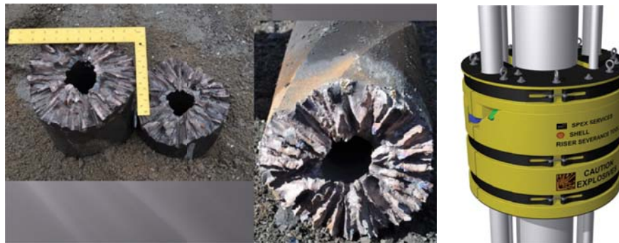
Figure 10.9: Sheared Pipe Using RST & RST Assembled on the Riser and Auxiliary Lines [40]
