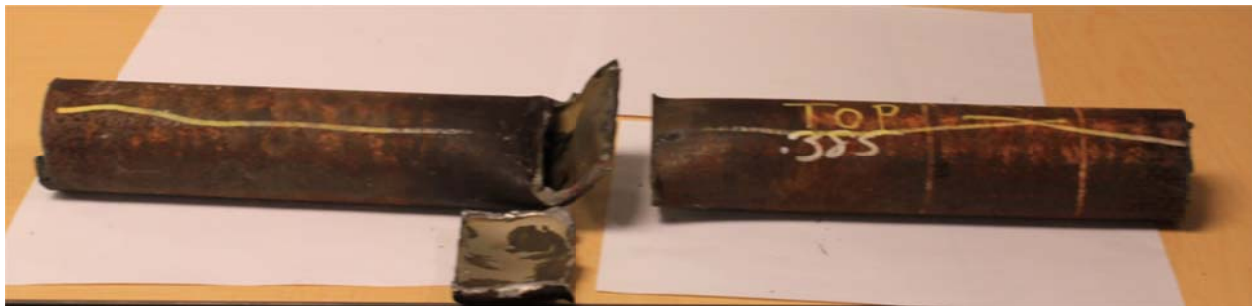
Figure 6.11: Shear Test 2 (Lower and Upper Fish, Front View)
