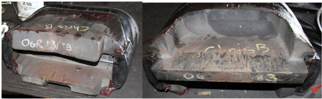
Figure 6.20: Upper and Lower Shear Ram Used in Shop Test
