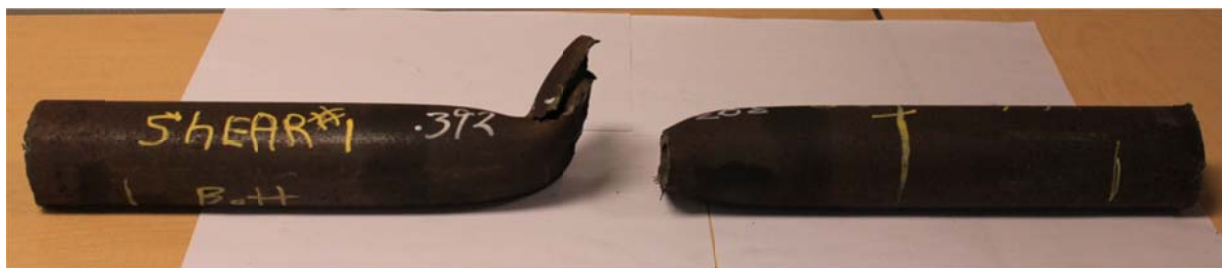
Figure 6.9: Shear Test 1 (Lower and Upper Fish, Front View)
