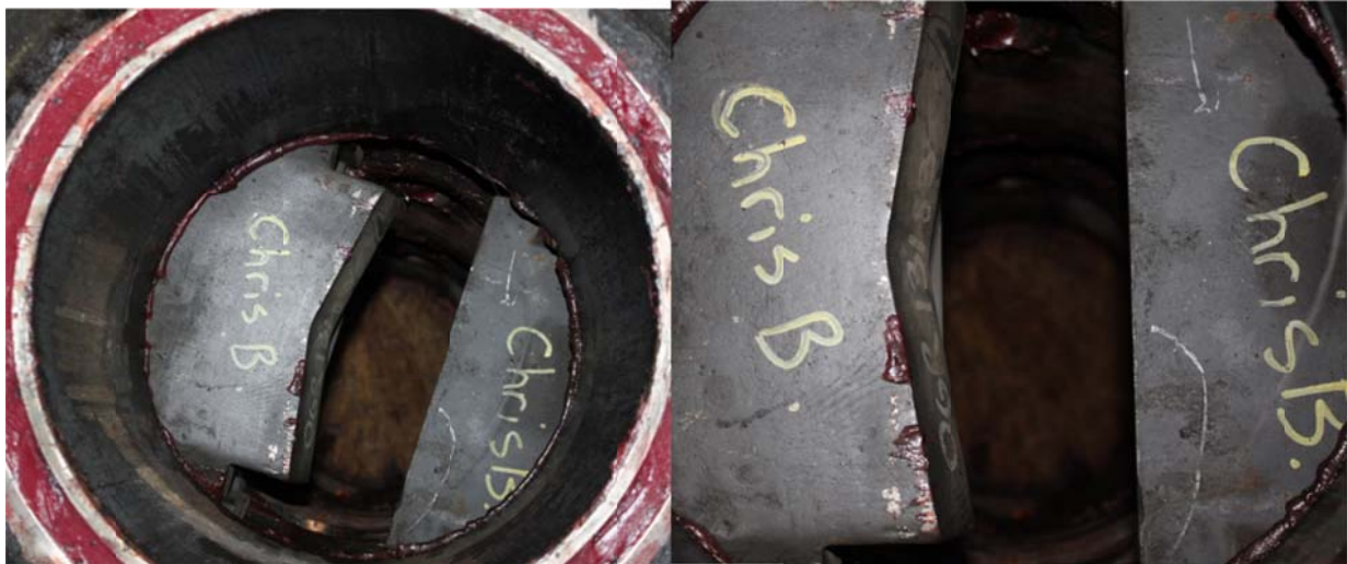
Figure 11.1: Condition of the Bonnet and Shear Rams Before the Test
