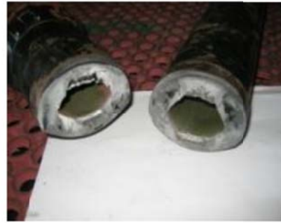
3.5"135S Pin-Box Connection) 4.4 O.D x 2.00 I.D Cutting Pressure 4957 psi
