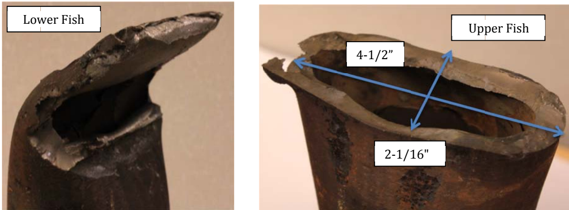
Figure 6.10: Shear Test 2 (Lower and Upper Fish, Close Up View)
