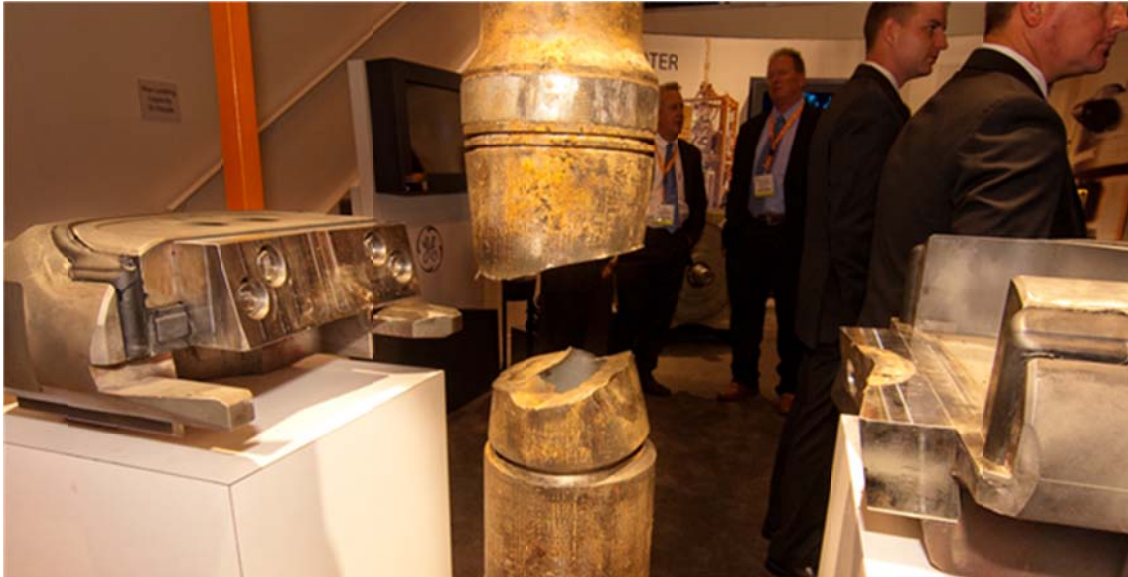
Figure 8-3: GE 5k Blind Shear Ram [33]
