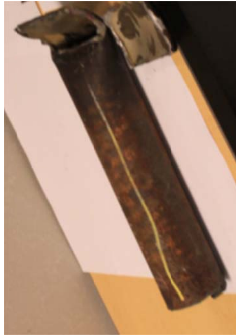
Figure 6.39: Sheared Drill Pipe in Test 2: Bottom Fish
