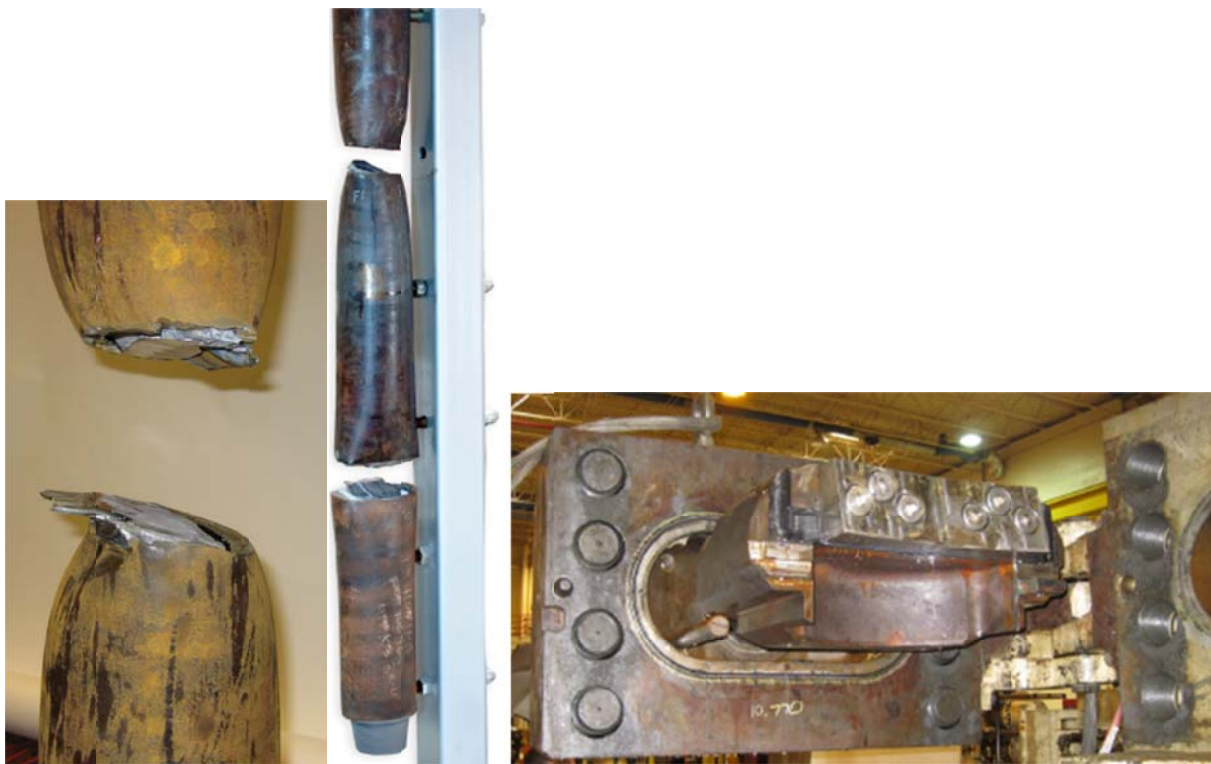
Figure 10.10: Sheared Drill Collar and Shear Ram Used for Testing [43]
