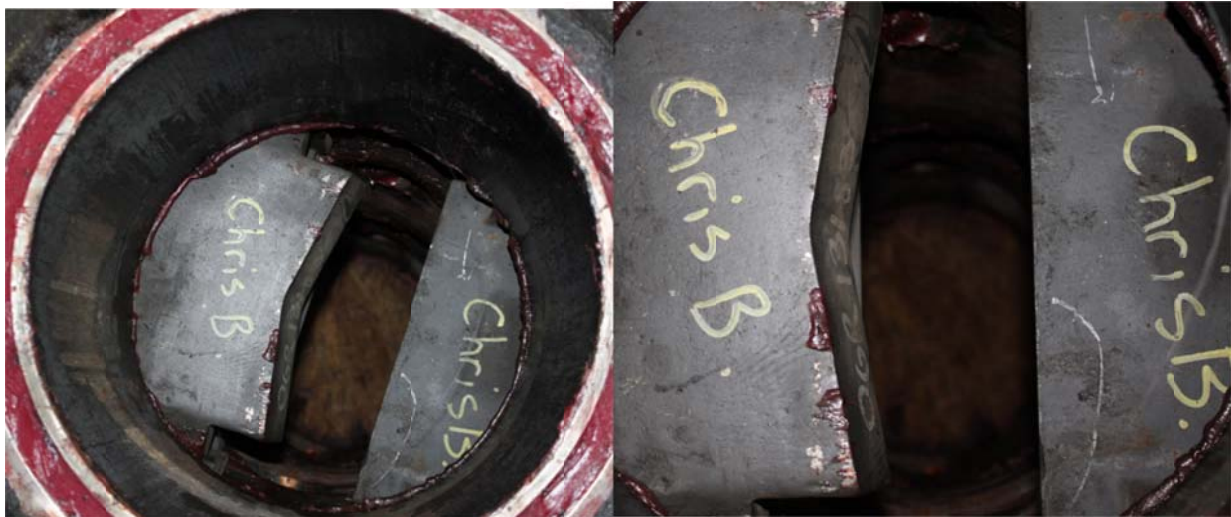
Figure 6.4: Condition of the Bonnet and Shear Rams Before the Test
