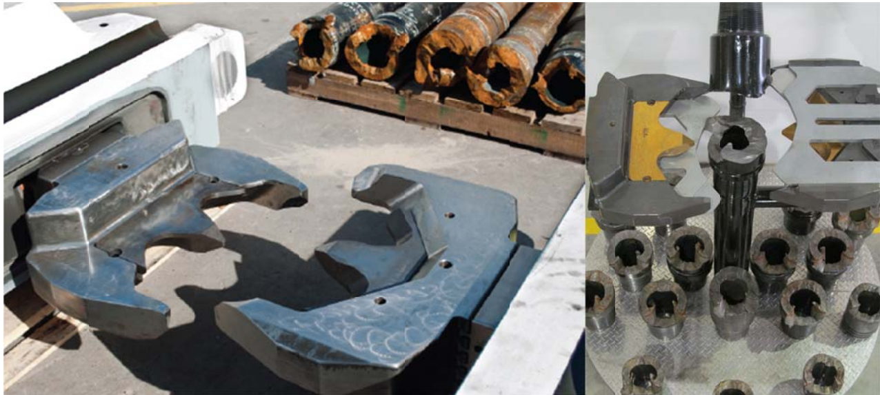
Figure 8-1: NOV Low Force Shear Ram [25]
