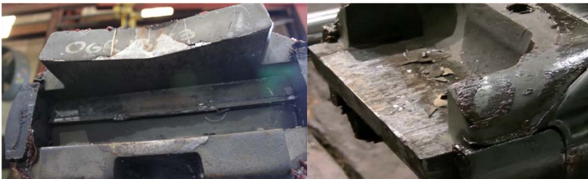
Figure 6.12: View of Upper and Lower Shear Rams After the Test
