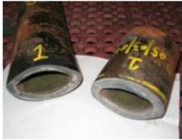
3.5"15.5 ft/lbs S135 Drill Pipe Upset Cutting Pressure 3133 psi
