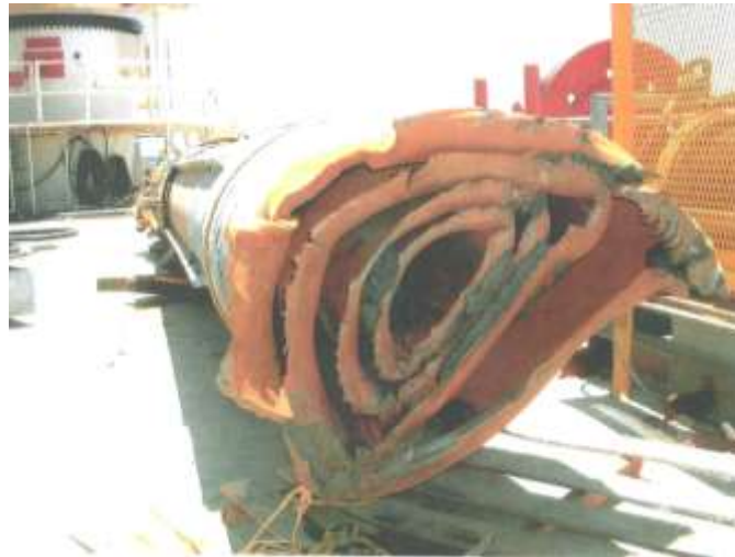
Figure 6-24. Multi-string Conductor Sheared below the Mudline (Photo courtesy of Prime Marine Services, Inc.)
