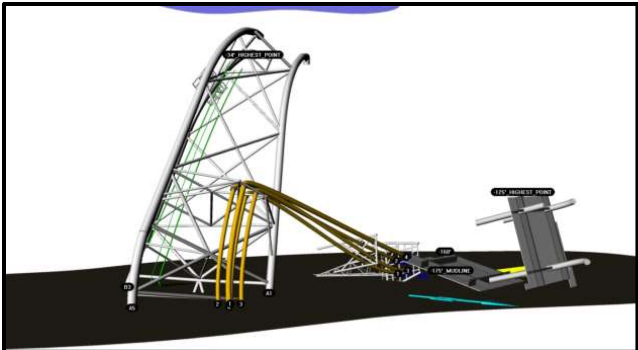
Figure 5-12. Damaged Vermilion 281-A Platform, 2008
