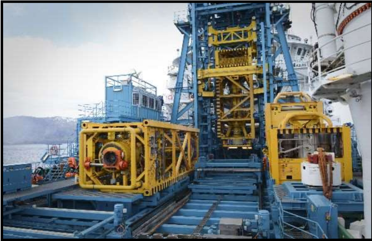
Figure 6-12. Expro Group AX-S Subsea Well Intervention System (Photo courtesy of Expro)
