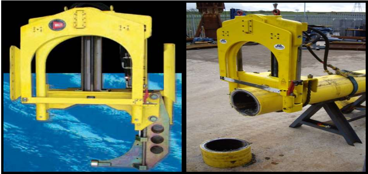
Figure 6-19. Guillotine Saw (Courtesy of EH Wachs)
