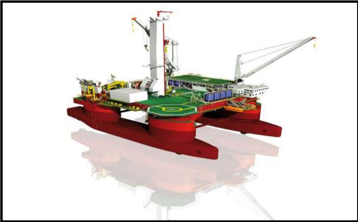
Figure 6-10. Q4000 Well Intervention Vessel (Drawing courtesy of Helix Energy)
