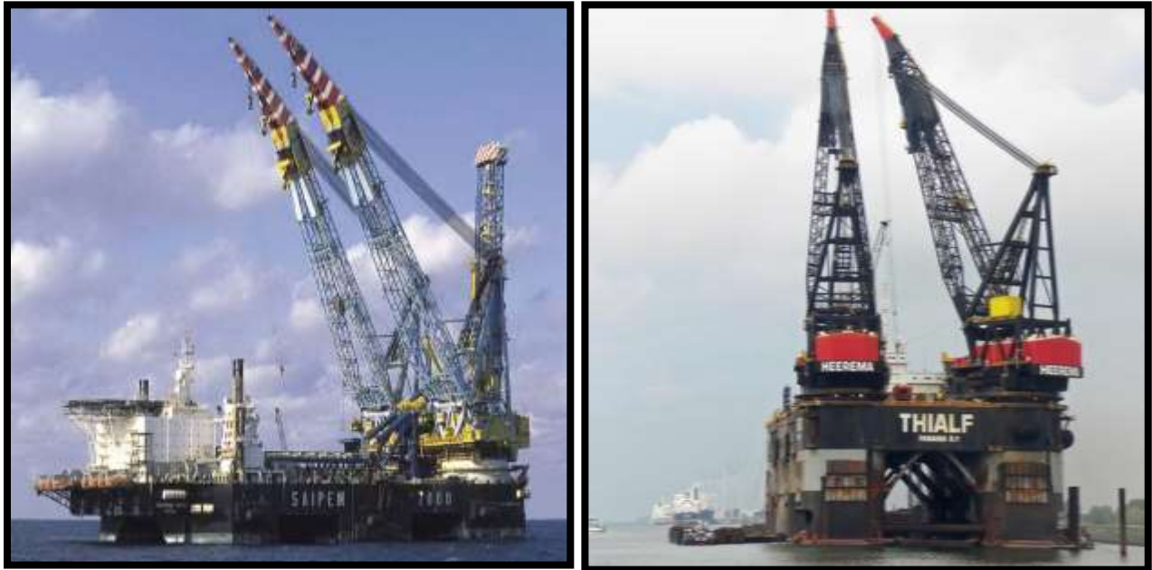
Figure 6-29. Siapem 7000 and Heerema Thialf Semi-Submersible Crane Vessels (Photos courtesy of Saimpem and Heerema)
