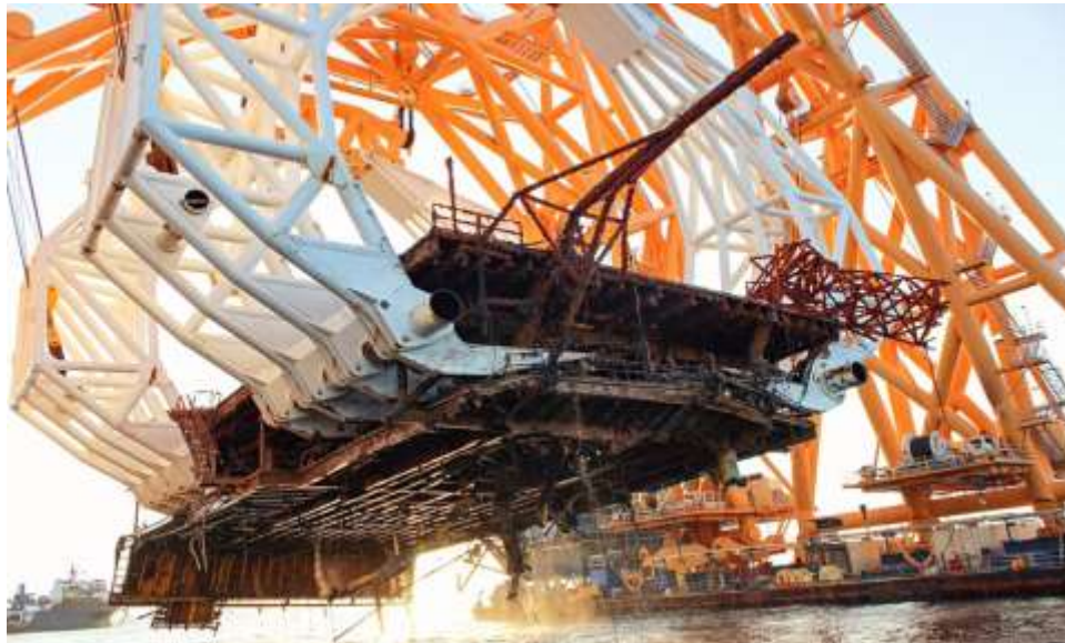
Figure 6-34. Versabar Claw Controlled by VB 10,000 Lift System (Photo courtesy of Versabar)
