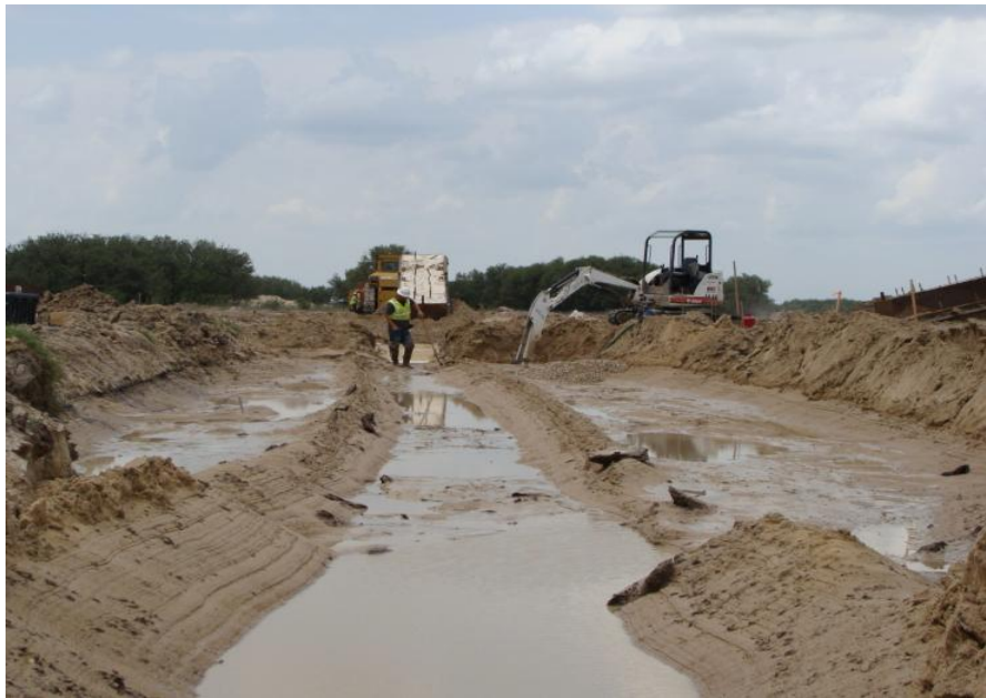
Figure 4.9: Typical Gouge Produced in Sand Test (Sancio et al., 2011 [38])
