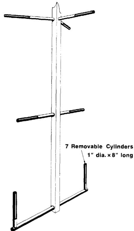
Figure 4. Array of ice accretion measurement cylinders.
