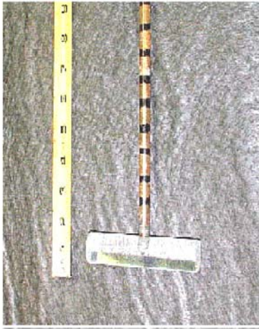
Fig. 6 Tee-Bar Used to Estimate Undrained Shearing Strengths
