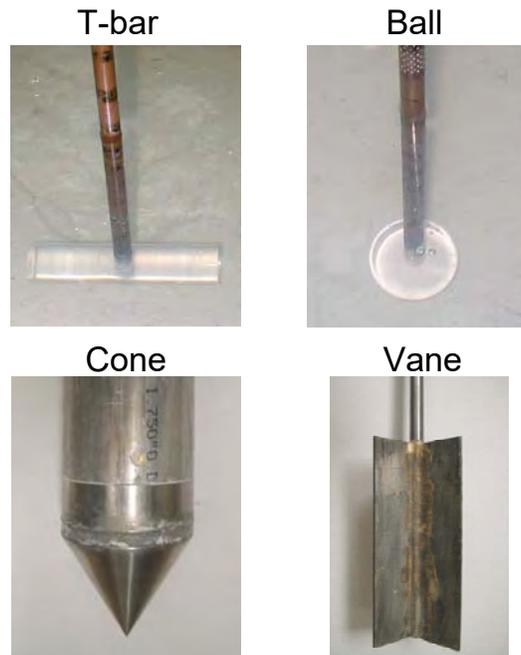
**Figure 4. Methods of in-situ shear strength measurement**
