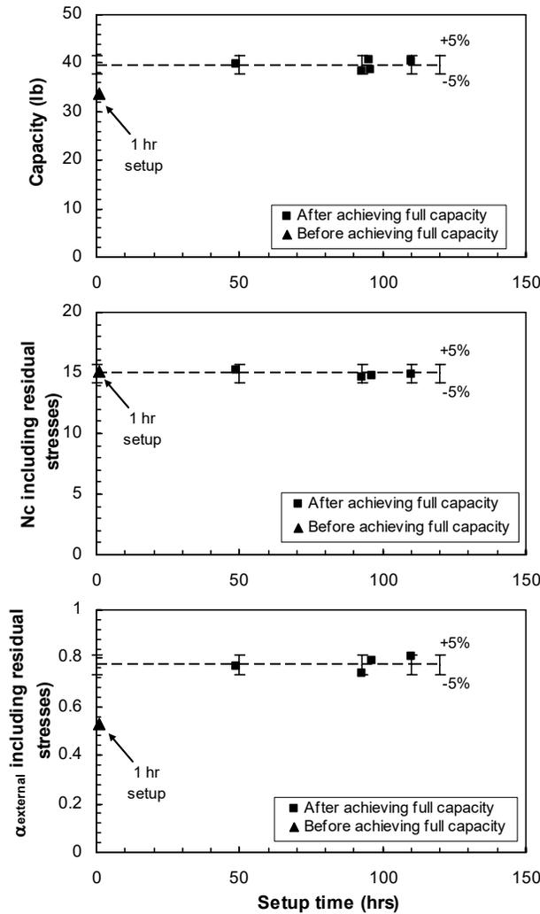
Figure 16. Effect of the setup time on the (a) capacity, (b) end-bearing resistance, and (c) the external side friction of the double-walled caisson during pullout with a sealed top
