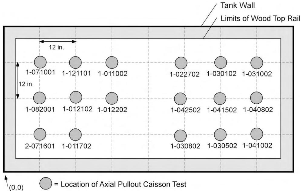
Figure 8. Test Locations in Test Bed 1 (Luke, 2002).
