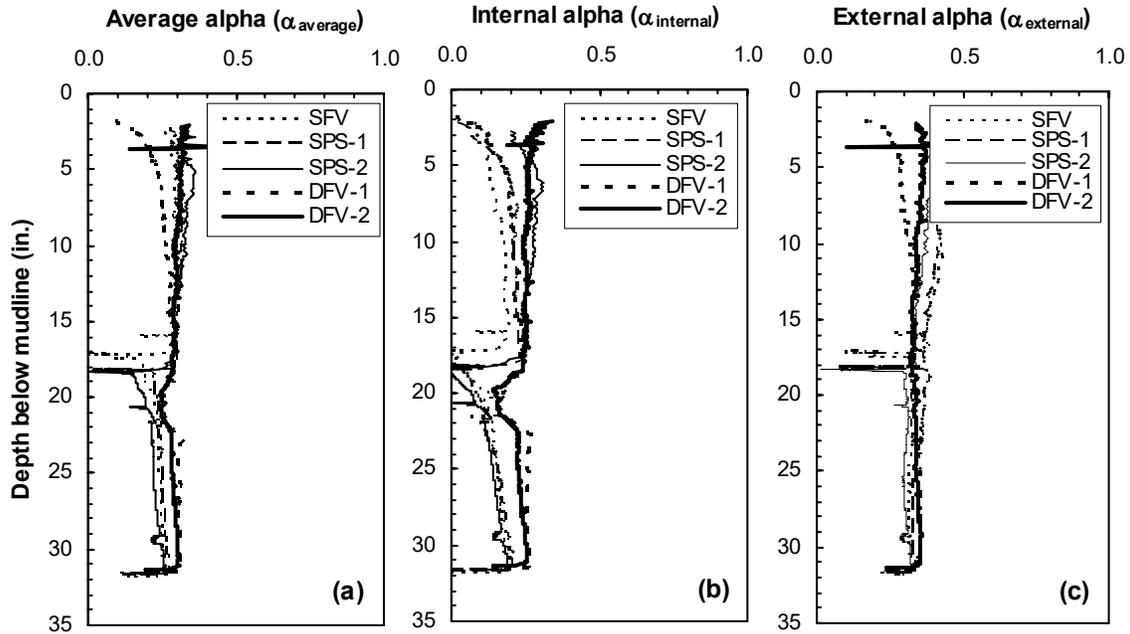
**Figure 15. Alpha factors back calculated form insertion of the double-walled caisson in test bed 4: (a) average alpha, (b) internal alpha, and (c) external alpha (Note: test ID starting with S indicates suction insertion, while test ID starting with D indicates deadweight insertion)..**
