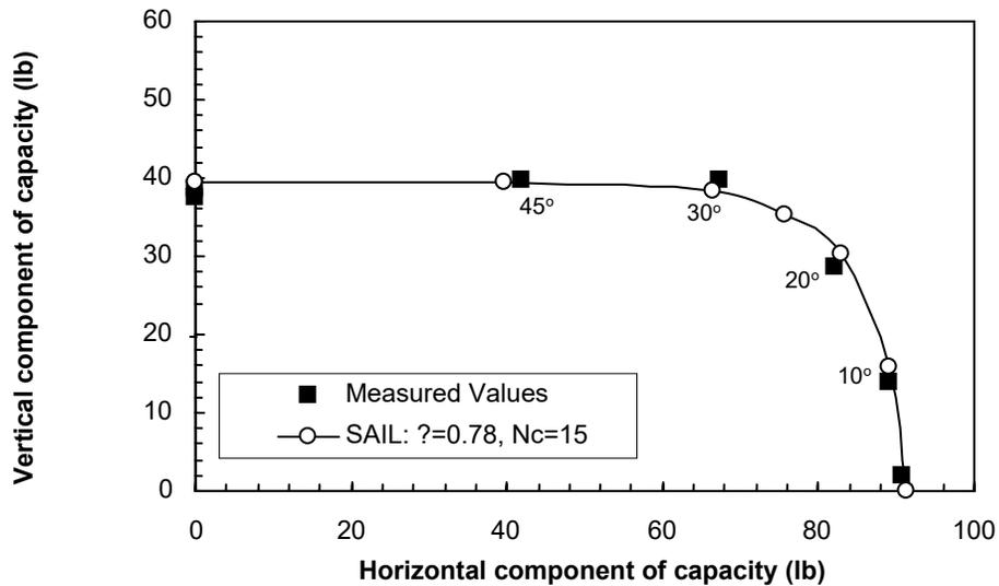
**Figure 13. Comparison between measured and predicted components of the suction caisson capacity under inclined loading.**
