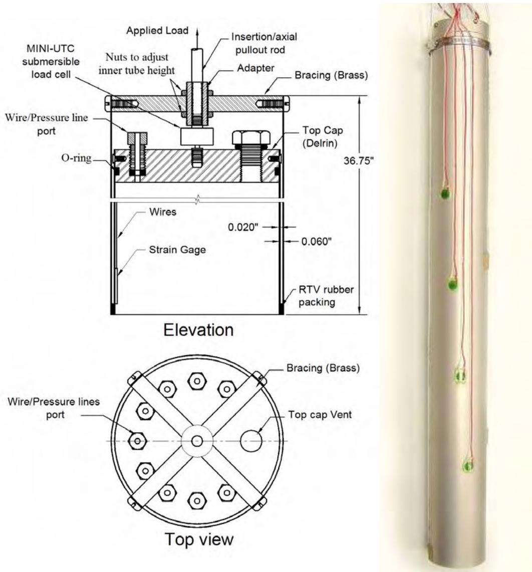
Figure 7. Conceptual diagram of the double-walled caisson.
