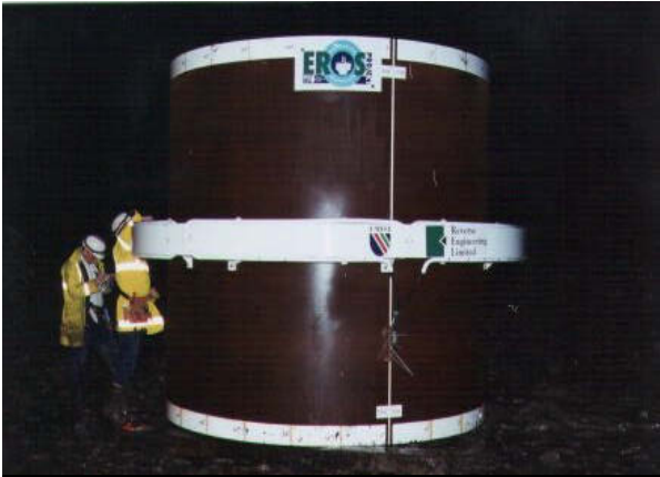
Photo 25. Charge assembled on 10 Foot OD Tubular
