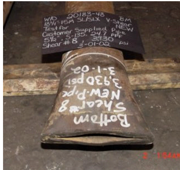
Figures 3.1 and 3.2: Example shears of low ductility or brittle pipe (left) and high ductility pipe (right). The high ductility pipe required almost 2,000 psi (over 300,000 lb) more to shear than the low ductility pipe even though the grades on both pipes were the same, S-135. Visual differences in the shears can also be easily noted: the brittle pipe on the left has cracking on the sides and did not collapse as much as the more ductile pipe on the right. The ductile pipe had no cracking on the sides. In the severest of cases, very brittle pipe cracks considerably when being collapsed by the shear rams and then requires less force to complete the shear.
