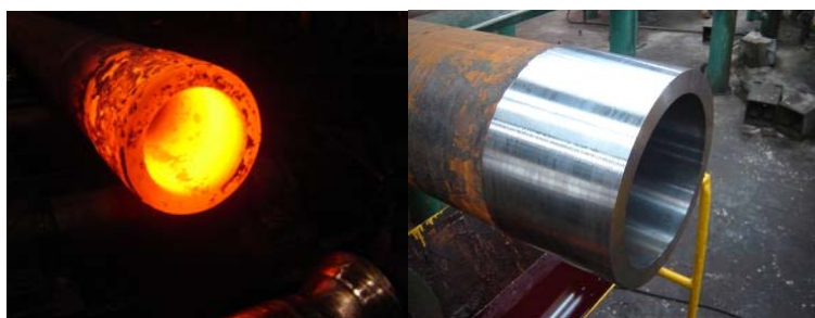
Figure 7.1. Steel Pipe as Upset and as Machined – GOM Design Case
