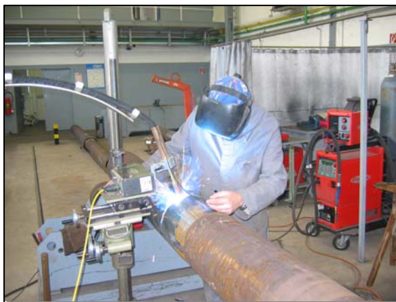
Figure 7.5. Welding Using Mechanized GMAW (Source: SZMF, Duisburg)
