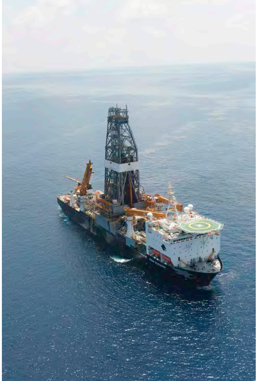
This dynamically positioned drillship, the Ocean BlackHawk, is capable of operating in water depths up to 12,000 feet and can drill to a depth of 40,000 feet. Owned and managed by Diamond Offshore Drilling, the Ocean BlackHawk is currently operating in the Gulf of Mexico.
